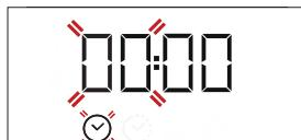
Use + or - to set the hour and press
